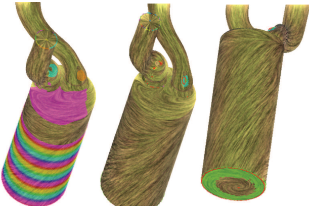
Fig. 13. A comparison of the obtained Morse sets of the diesel engine simulation data set. The first image shows the Morse sets obtained using the geometry based mapping. The two images to the right show the result using a multi-valued map with d_\epsilon = 1 from two different view points. Note how much more refined the topological regions become.
